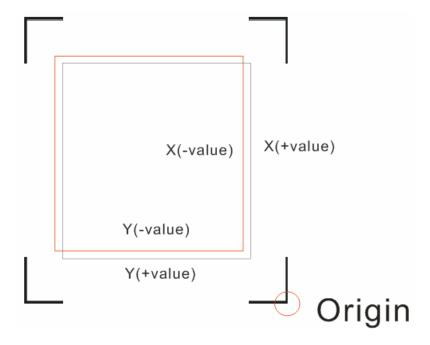
The red line is the position of the real cutting, the offset value of the red line and the printed line is X=0.4, Y=0.4, the new canculated value is DX=-0.3+(-0.4)=-0.7, DY=0.5+(-0.4)=0.1
