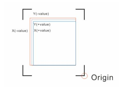
Black line is the original image, the red and the blue line is the actual figure drawing. the origin is alignment, but up-left is not, Parameters of BX and BY the value of the need to adjust.
