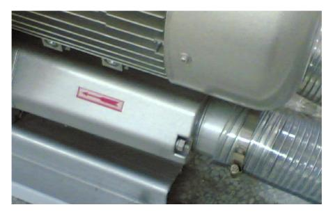
Pipe connection, there are 2 or 4 pipe connectors under the pump. Connect the 50mm flexible pipe, and lock it with steel hoop.
