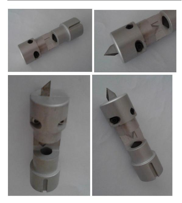
Tangent knife holder installation: insert the holder into the tool fixer. (Attention: the socket on the top of tangent knife holder should correspond to the inside sign of tool fixer, or also can correspond to the tool fixer.)
