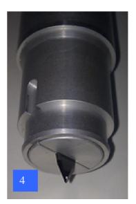
Knife set holder installation: the purpose to install knife pouch is to make the material which is easy turn-up well fixed on the table during high speed cutting, make the sign on the knife pouch and socket of the tool fixer to align, then insert knife set.
