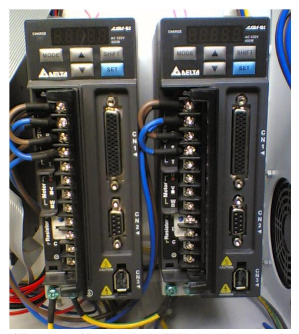
3.Y motor power and X motor encoder wire, U,V,W and earth wire are connected to the corresponding terminals of Y driver motor. The connector of encoder will be connected in the socket CN2 of Y driver motor.
