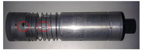
Install the tangential tool in the head: unlock the retaining ring on the top of the head, unlock to make the retaining ring to be even with knife holder, and make the
