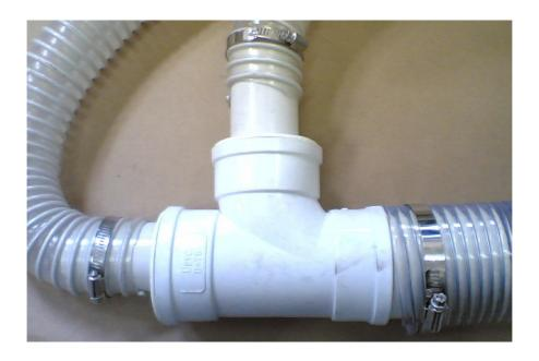
Connect the silencer to the pump outlet with a shorter diameter of 75mm.
