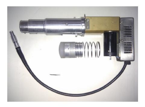
Oscillating knife installation: unscrew the inside hex screw in the direction of oscillating knife head, insert the oscillating knife into the bottom of the holder and then screw up the hex screw.
