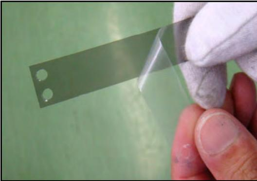
6. Peel off the left end of the protection film on the new linear encoder scale.
