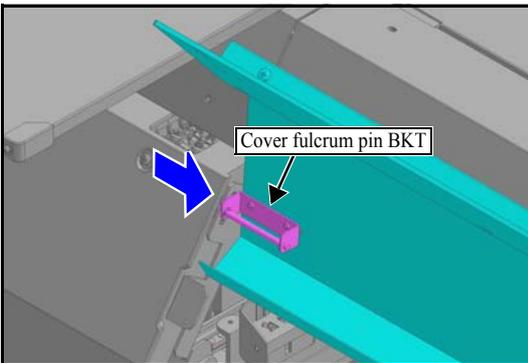
2. Shift the cover fulcrum pin BKT to right, and remove the **front panel cover M**.
