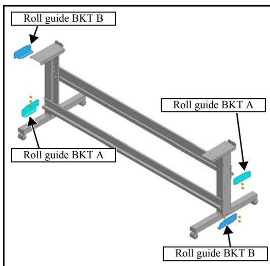
3. Fix the **roll guide BKT A/B** to the leg with the 10 screws (M5x15).
