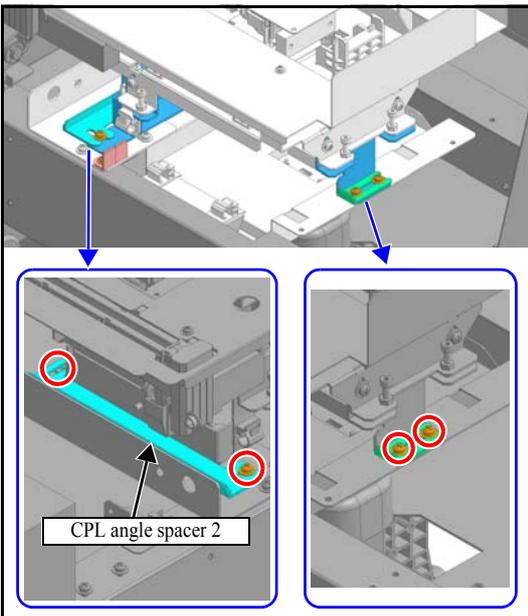
7. Loosen the four screws in the left figure.
