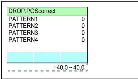
9. Correct the dot positions for pattern 2 onwards in the same way as Step 6, then press the [ENTER] key.
