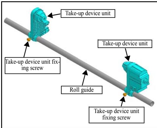
6. Put the **take-up device units** on the roll guide, and tighten the **take-up device unit fixing screws**.
