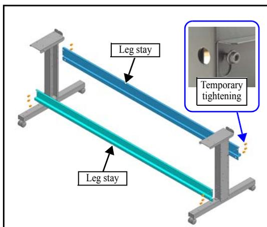
2. Fix the **leg stay** to the leg with the 12 screws (M5x15).
