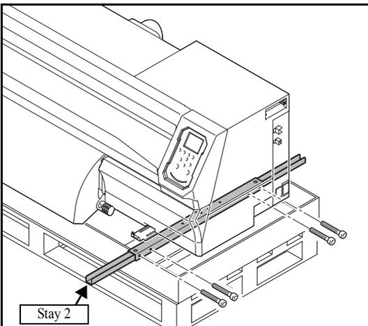
12. Using the 8 screws (CS6x55 Black), attach the **Stay 2** to the Stay 1.
