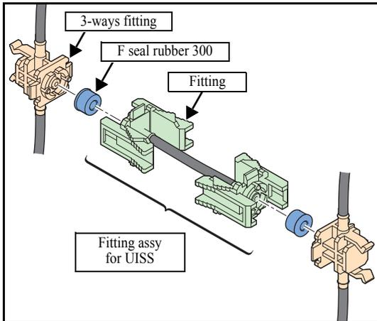
2. Release the knob of fittingφ2, and remove the **fitting assy for UISS**.
