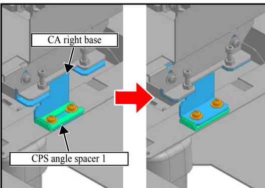
8. Pull out the **CPS angle spacer 1**.
