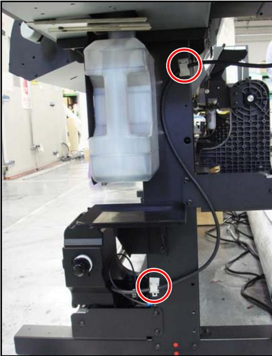
23. Fix the cable of the take-up device unit with the cable clamps (x2).
