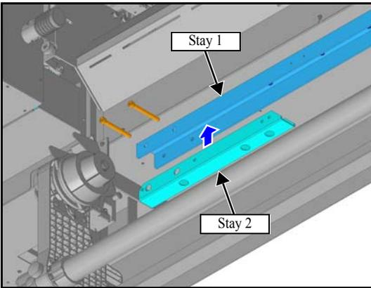
3. Using the screws (CS6x55 black x4), attach the extra **stay 2** to the stay 1.
