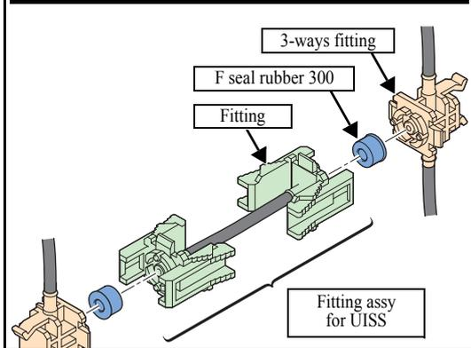
8. Attach the **F seal rubber 300** removed in the procedure 6 and the new **Fitting** to the 3-ways fitting.
