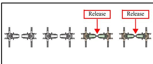
7. Release the knob of fitting $\phi$ 2, and remove the **fitting assy for UISS**.
