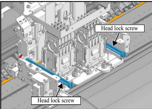
9. Tighten the **head lock screw** with a standard screw drive or a coin.
