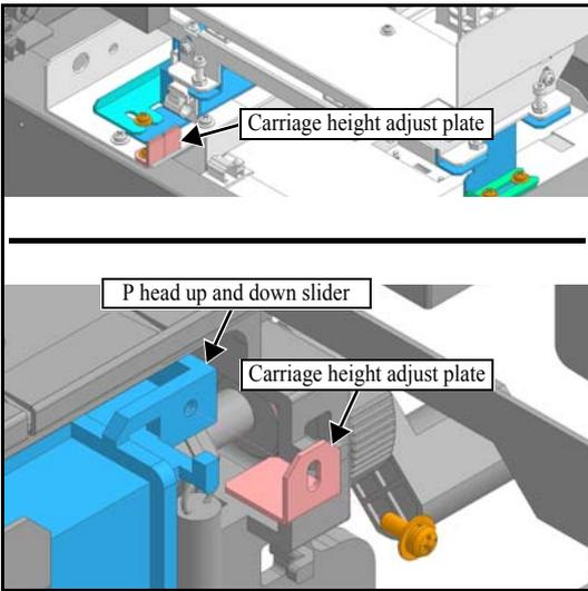
8. Remove the **carriage height adjustment plate**, and attach it to the **P-head up and down slider**.
