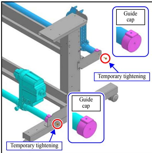
7. Fit the **guide caps** on both sides of the roll holder assy and the take-up device assy, then temporarily tighten them with the 4 hexagon socket head screws (SSWP4x4(R)) (such that the screw touches the roll guide).
