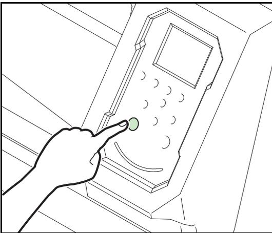
2. Turn the power on, by pressing the [END/POWER] key.
