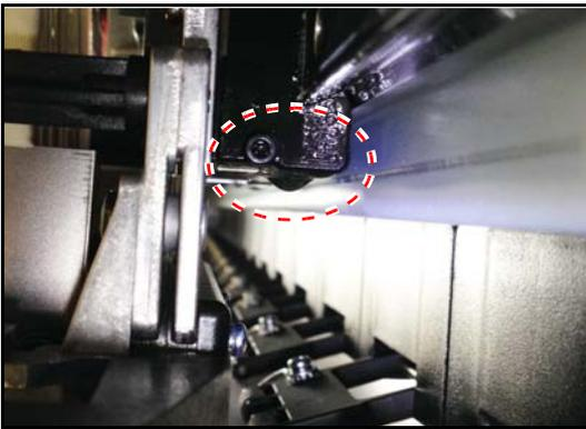
2. Visually check the LM guide left/right ends and the LM guide block unit for formation of grease droplets, and wipe away any grease droplets.
