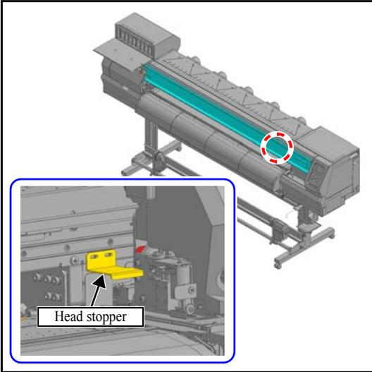
1. Open Front cover, remove the 2 screws (P3x8SMW), and remove **head stopper**.
