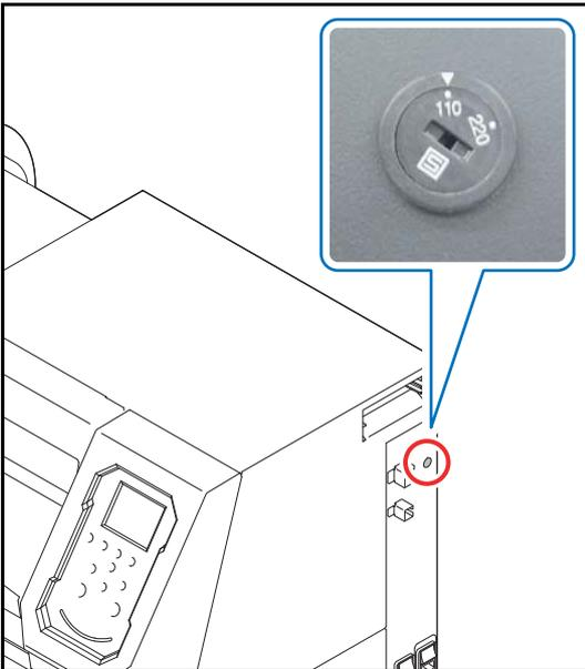
1. Switch the voltage selector switch to the side for the voltage you are using.
