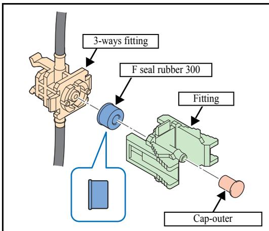
3. Attach the **F seal rubber 300** removed in the procedure 2 and the new **Fitting** to the 3-way fitting.
