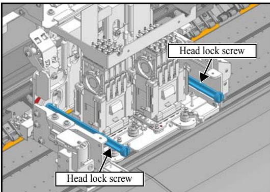
7. Loosen the **head lock screw** with a standard screw driver or a coin.
