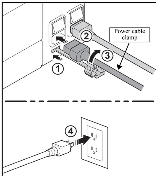
1. Insert the **power cable clamp** into the power supply box.
