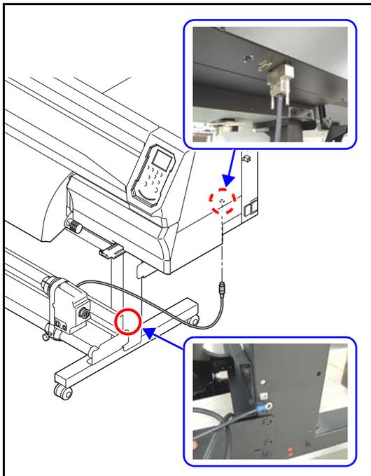
21. Insert the cable of the take-up device into the connector on the bottom surface of electric unit.
