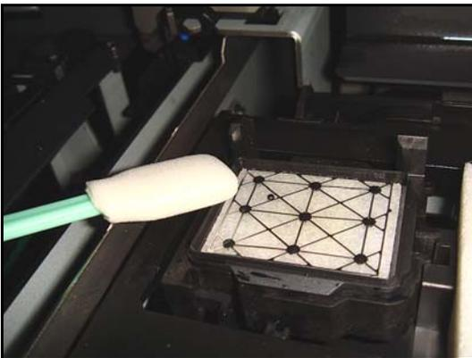
1. Dip the clean stick into the washing solution, and moisten the edges of cap.
