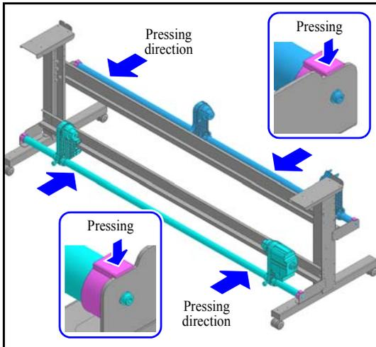
8. While pressing the **roll holder assy** and the **take-up device assy** towards the leg stay, affix the **roll guide BKT**.
