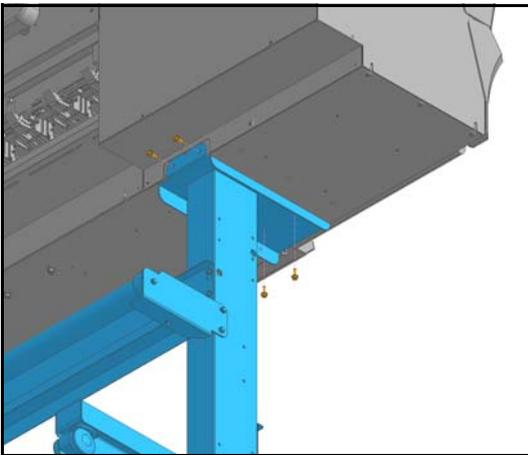
15. Fix the main unit and legs with the 8 screws (M5x15).
