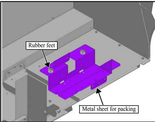
1. Attach the **metal sheet for packing** and the **rubber feet** on the back surface of main unit with the screws (P4x20 SMW x 4).
