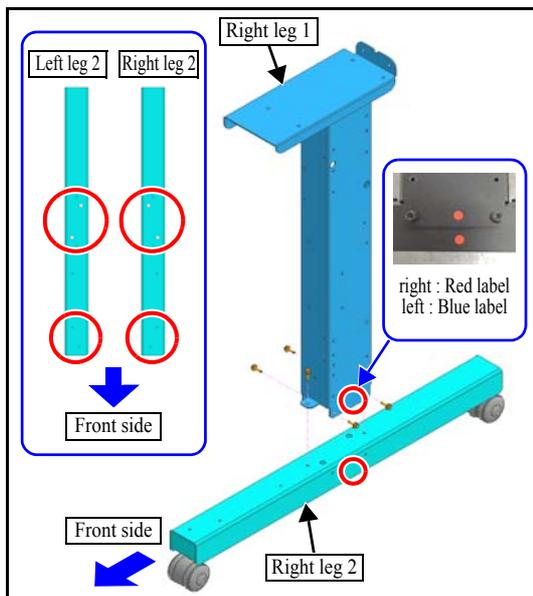
1. Fix the **right leg 2** to the **right leg 1** with the 6 screws (M5x15).
