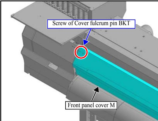
1. Loosen the screw of **cover fulcrum pin BKT** which is at the left side of front panel cover M.
