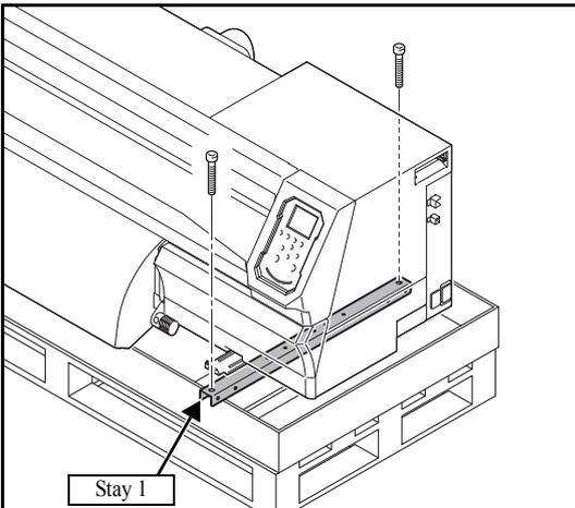
11. Remove screws of the **Stay 1** of both sides of the Main unit.
