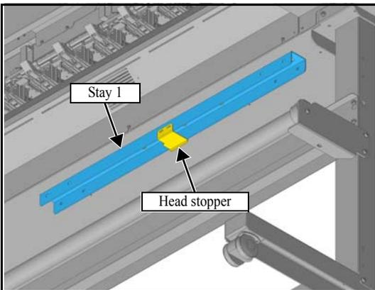
4. Attach the **head stopper** to the stay 1 with the screws (P3x8 SMW x 2).
