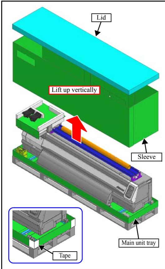
1. Remove the **lid** and **sleeve** of the box packing the main unit, cut the tapes stuck on 4 corners of the **main unit tray**.
