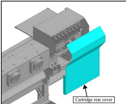
6. Remove **cartridge rear cover** from the back panel of the main unit.
