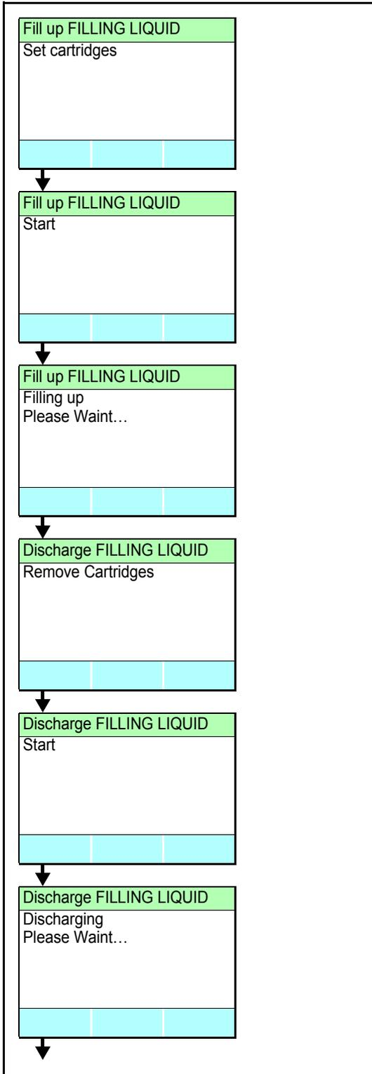
10. Set the filling fluid cartridge, and press [ENTER].
