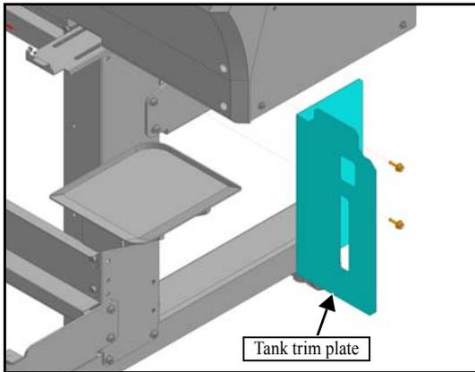
6. Attach the **tank trim plate** to the right leg with the 2 screws (M5x15).
