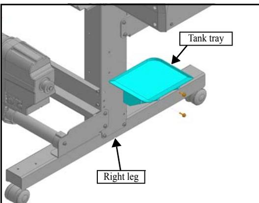
5. Fix the **tank tray** to the right leg with the 2 screws (M5x15).
