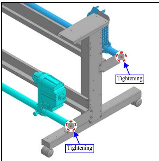
9. Tighten the 4 hexagon socket head screws (SSWP4x4(R)) that were temporarily tightened on the [step 7](#). (Tighten the screw 90°angle once it hits the roll guide.)
