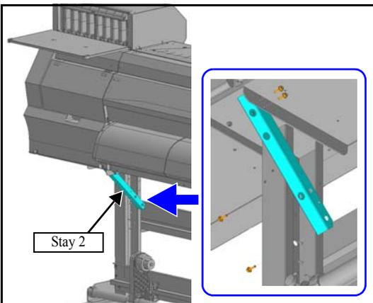
4. Fix the **stay 2** to the screws (M5x15) being used on the stay.
