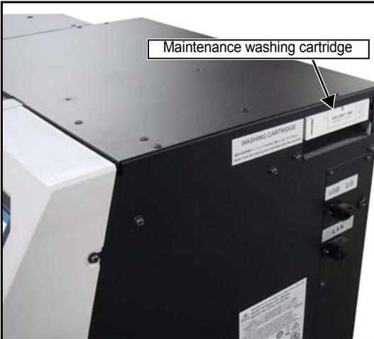
15. Set the removed filling maintenance washing cartridge to the washing cartridge of the right side of main unit.
