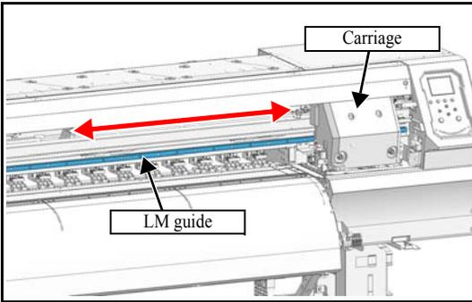
1. Using manual operation, move the carriage back and forth along its full travel distance several times.
