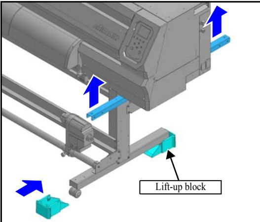
1. If the installation location is decided, lift up the main unit by the stay, and put the **lift-up block**.
