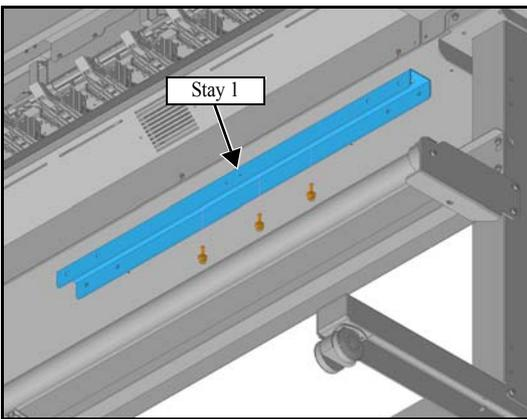
2. Attach the **stay 1** on the back surface of main unit with the screws (CS6x20 SMW x 6).
