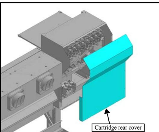
1. Remove **cartridge rear cover** from the back panel of the main unit.
