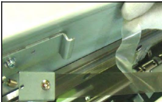
8. Mount the **Scale holder L** on the **Linear encoder scale** so that the surface where the protection film is stuck faces to the Y bar side.
