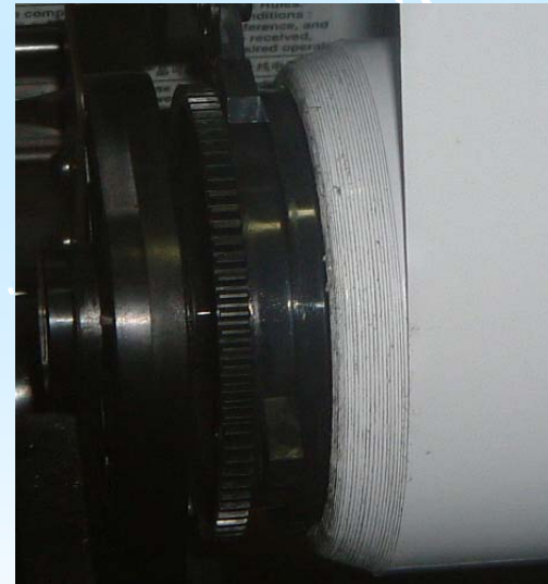
Pyramid edges on feed roll
