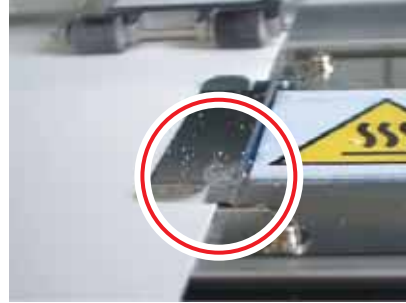
Metal paper guide with dust
