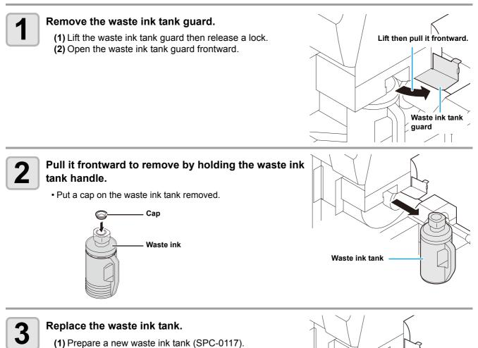
(1) Prepare a new waste ink tank (SPC-0117). (2) Insert the waste ink tank by holding a handle of the tank.
