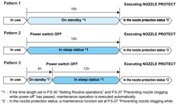
power-off" does not work. After entering the nozzle protection status, this machine automatically performs NOZZLE PROTECT regularly.
