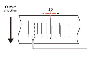
The dots at the fourth position counted from the zero position in the positive direction form a straight line. In this case, the dot position correction value is 4.0.
