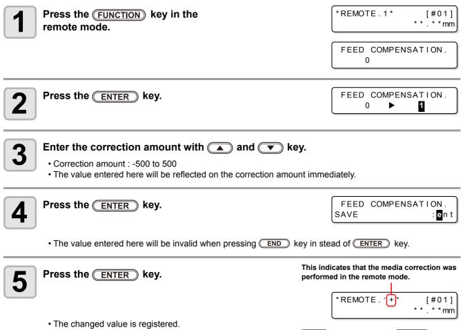
• The value entered here will be valid temporarily when pressing **END** key in stead of **ENTER** key. (If performing media detection again or turning OFF the power supply, the correction value will be cleared.)
