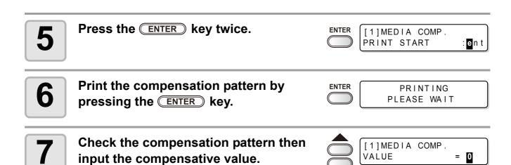
Input to " + " : Move to such direction that a spacing between two lines is getting wider. Input to " - " : Move to such direction that a spacing between two lines is getting closer.
