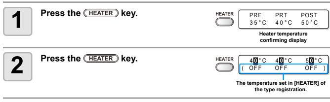
3 Set the temperature of each Heater by pressing the keys.
