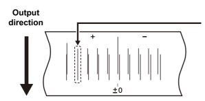
The dots at the fourth position counted from the zero position in the positive direction form a straight line. In this case, the dot position correction value is 4.0.
