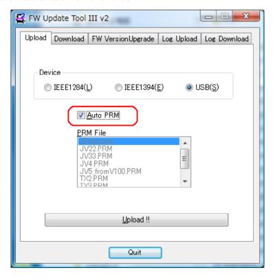
Auto PRM function is the function users can upload and download parameter without PRM file settings by PC. The product's firmware needs to be corresponded to the function.
