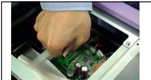
1. Pull out the **head FFC assy** and **head memory cable assy** from the **ink slider PCB assy** through the top where the wiring cover removed.
