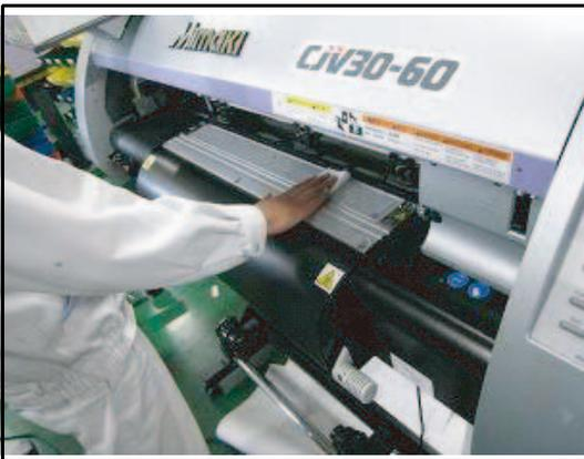
1. Remove oil on the platen with ethanol or diluted mild detergent.
