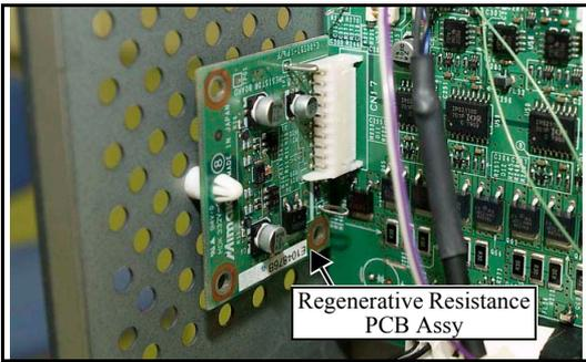
4. Draw the **regenerative resistance PCB assy** out of the main PCB assy.
