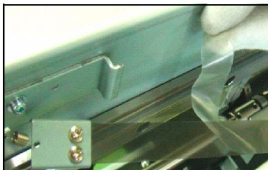
8. Engage the **scale hook** with the **scale base L** through a spring, and mount the **linear encoder scale** on the scale base R while peeling off the protection film.
