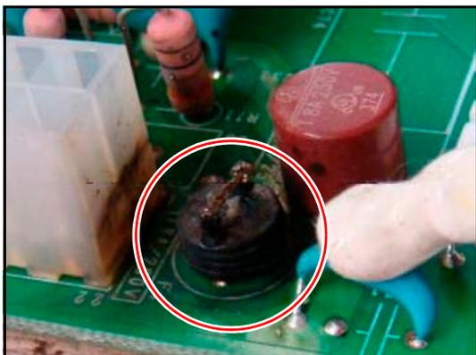
4. Check F4 and F5 of the power supply PCB.
