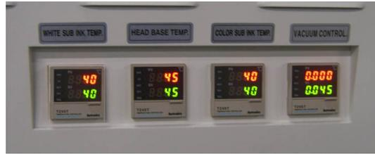
While warming Up, perform a number of (5) circulation cycles for the White in order to rinse the white ink tubes and to keep away any sediments from the heads.
