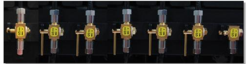
Perform a Purge of the Black head (with intervals of 2 seconds ON and 4 seconds OFF) till ink is coming out of the print heads. Do not purge when Sub Ink Tank is empty. After that purge all the other heads color by color.
