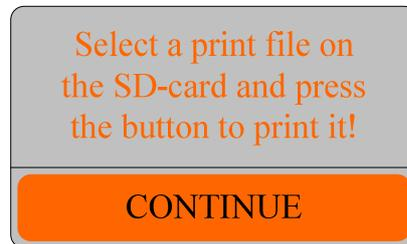
The display shows the files in SD-card. Rotate the button to select the file you would like to print. Then click the button to confirm the selcetion.
