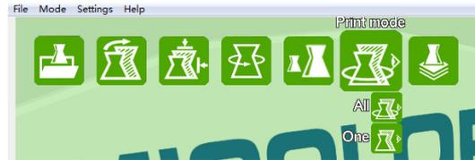
When [One] button is available, the 3D models in printing area will be sliced one by one. The generated Gcode can make them printed separately.
