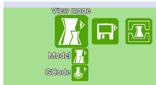
After models have finished slicing, selecting [GCode] shows the Gcode view.
