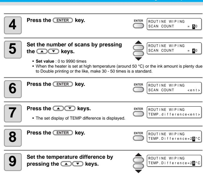
• The ROUTINE WIPING function is activated when the setting temperature of the print heater is higher than the ambient temperature and the difference is larger than the value of "TEMP.difference".
