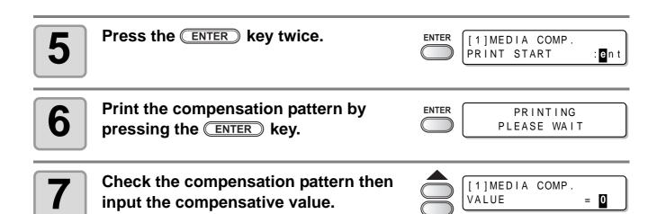
Input to " + ": Move to such direction that a spacing between two lines is getting wider. Input to " - ": Move to such direction that a spacing between two lines is getting closer.
