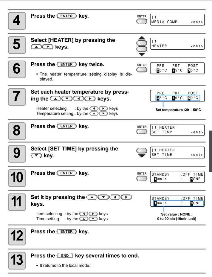
• Use this machine at 20-35 °C to ensure reliable printing. The heater temperatures may not rise to the set values depending on the ambient temperature.
