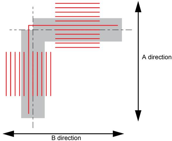
Misaligned by +0.2 mm from the center line of the register mark (---) in the A and the B direction.
