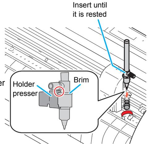
**7****Turn the knob clockwise to fix the tool.****2**
