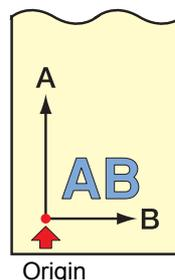
• After the sheet detection, the carriage will stop at the origin.
