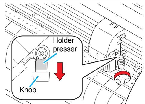
**6****Insert the pen adapter with the pen into the tool holder.**
