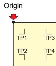
**7** Move the Light Pointer into the area shown below by pressing the appropriate ones of the jog keys ▲ ▼ ◀ and ▶ .
