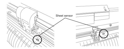
In the case where any of the following types of sheet is used, the sheet sensors will not be able to detect it to give the error message shown below.
