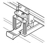
Low mode: Lower the clamp pressure lever.
