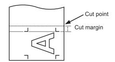
In case detected the distance from the TP2 and the TP1 registration mark during copying the registration mark continuously, cut off the sheet in between TP1 and TP2.
