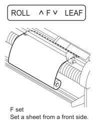
The device detects a sheet of media in the five different methods as shown below.
