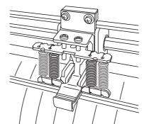
Low mode: Lower the clamp pressure lever.
