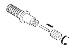
2) Exchange the cutter blade with tweezers.
