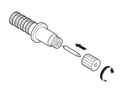
3) Tighten the cutter holder cap.
