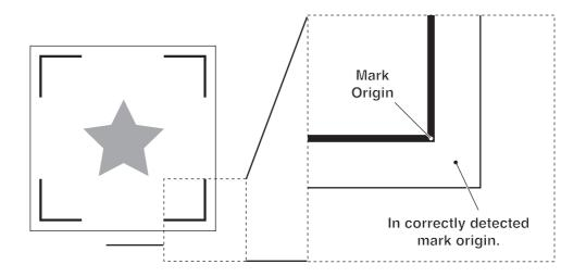
**Example of incorrect detection 2 :** The distance between registration marks(TP2&TP1, TP4&TP2) is smaller than the mark length (for TYPE2)
