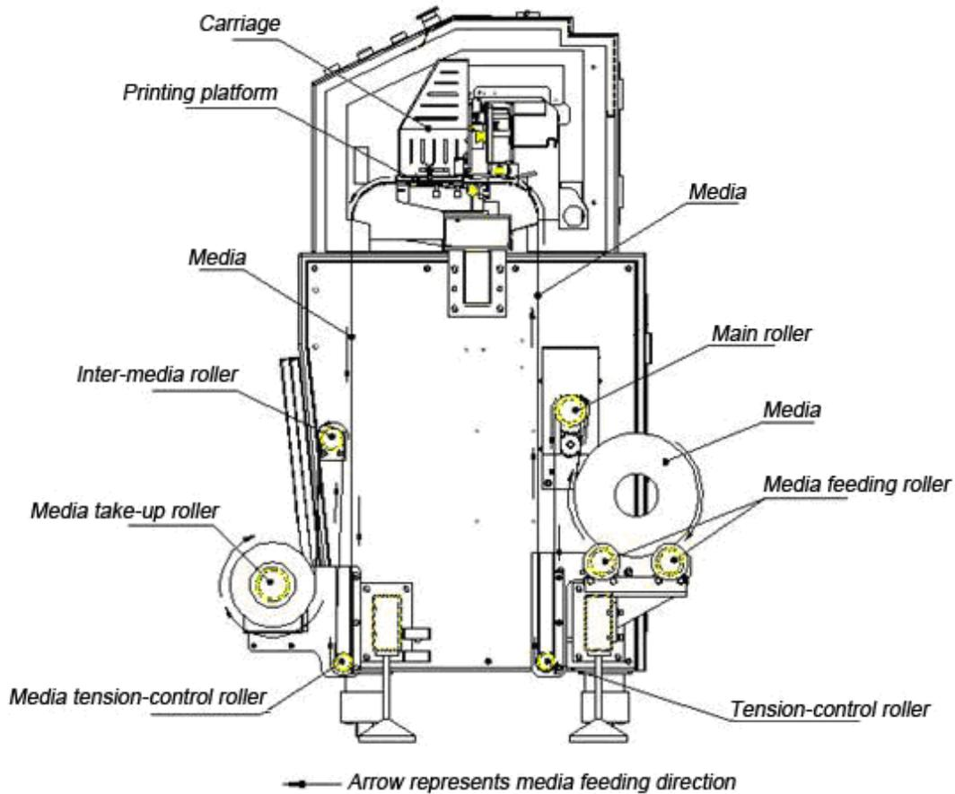
Lift up the lever, load the material according to the media track shown in the picture above onto the platform. Make sure media is aligned and smooth on platform. Tape the front edge of the media to the media roll up reel. Tighten the media on the media path by rotating the media roll to make sure no wrinkles on the media. Release the level.
