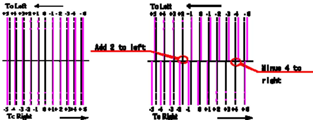
Read the number of the lines matched straight with black line in both printing directions. Add the numbers into the
