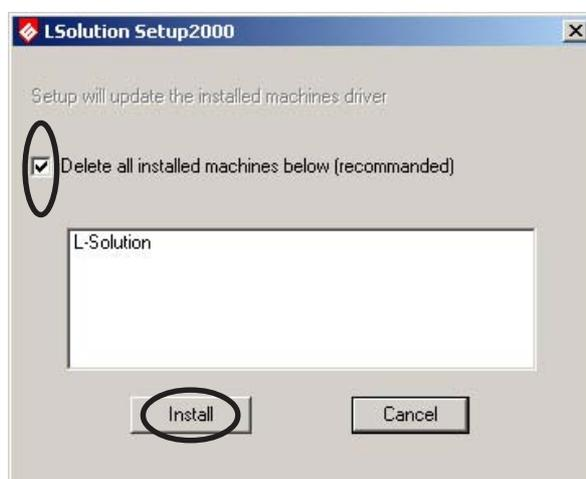
4. Seleccionar "Delete all installed machines below (recommended)" y pinchar en "Install".
