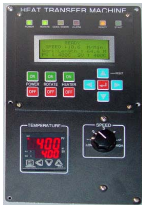
1 Zone Heater has one temperature controller
