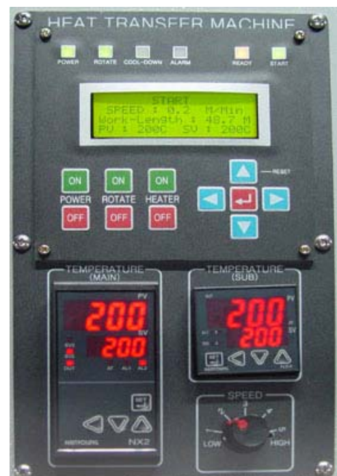
3 Zone Heater has 2 temperature controllers, one for the main heater, and one for the sub-heaters
