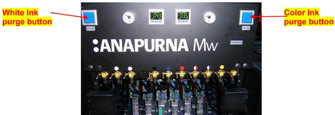
When purging too long, the ink refill system will not be able to keep up and the sub ink tanks may become empty. This may introduce air into the system. In order to check the condition of the sub ink tanks, verify the ink level indication in the main window of the control panel.
