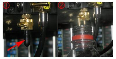
Close the mini-valve, remove the bottle and re-install all the parts.
