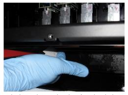
Clean the base plate with a dust free dry cloth. Or wetted with flushing solution
