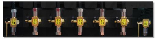
Pushing the Solution Valve Switch flush cleaning solution through the Black head. Than repeat this procedure color by color. Before pushing the Solution Valve Switch again check on the control panel the status of Solution (S=sub solution tank full, s=sub solution tank empty)
