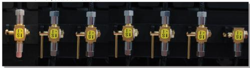
Perform a Purge of the Black head (with intervals of 2 seconds ON and 4 seconds OFF) till ink is coming out of the print heads. Do not purge when Sub Ink Tank is empty. After that purge all the other heads color by color.
