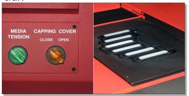
On the control panel press "ESC" to go Off-Line and than press "Capping Station" to move the shuttle to the capping station.
