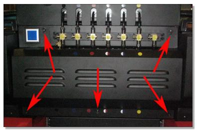
Remove the black cover from the mini-valve (1) and place it under it an empty bottle (2).
