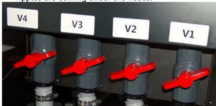
Air Valve position if all 4 compartments are fully covered (full width media).
